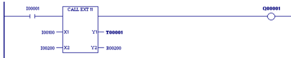
Figure 8: Calling an External Block in Ladder Logic
